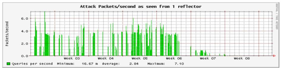
Assuming 4 KB TXT record we can extrapolate the bandwidth from the reflector, again consistent with avg reflector bps
